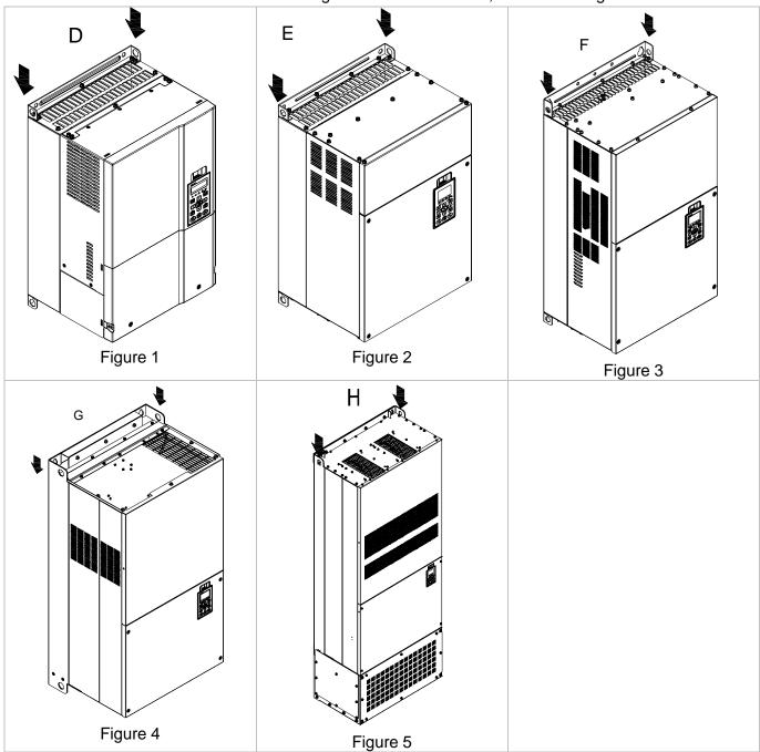
Ensure the lifting hook properly goes through the Ensure the angle between the lifting holes and the lifting hole, as shown in the following diagram. lifting device is within the specification, as shown in the following figure. (Applicable to Frame D~E) (Applicable to Frame D~E) >1/2 A (Applicable to Frame F~H) (Applicable to Frame F~H)
