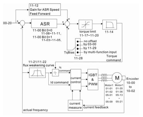
When setting Pr.00-11 to 5, FOC sensorless control diagram is shown as follows.
