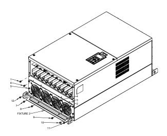
2. Loosen 12 screws and remove Fixture 2. Screw torque: 24~26kg-cm (20.8~22.6lb-in).
