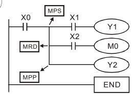
LD X0 Load contact A of X0 **MPS** Save in stack Connect to contact A of AND X1 X1 in series OUT Y1 Drive Y1 coil Read from the stack **MRD** (without moving pointer) Connect to contact A of **AND** X2 X2 in series OUT M0 Drive M0 coil **MPP** Read from the stack
