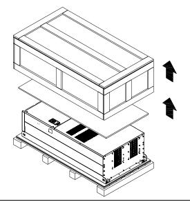
Loosen the 6 screws on the top then remove 6 metal washers and 6 plastic washers as shown in figure below.
