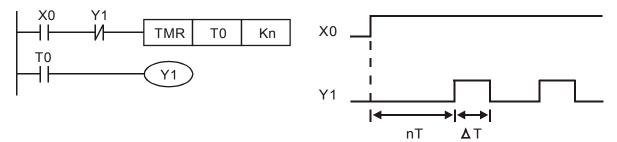
The figure above uses timer T0 to control coil Y1 to be ON. After Y1 is ON, timer T0 will be closed at the next scan period and output Y1. The oscillating circuit will be shown as above. (n is the setting of timer and it is decimal number. T is the base of timer. (clock period))
