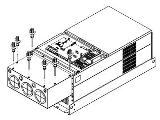
Place the cover back to the top and fasten the screws (as shown in the figure). Screw torque:  $12\sim15$ kg-cm ( $10.4\sim13$ lb-in).
