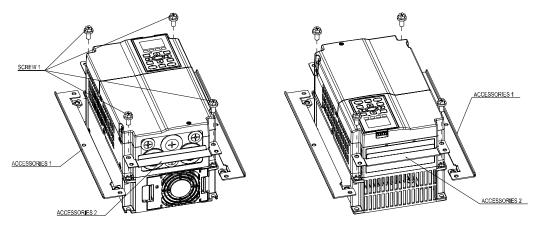
2. Plate installation, place 6 of the screw 2 (M6) through accessory 1&2 and the plate then fasten the screws. Screw torque: 25~30kg-cm (5.21~6.94lb-in). (As shown in the following figure)
