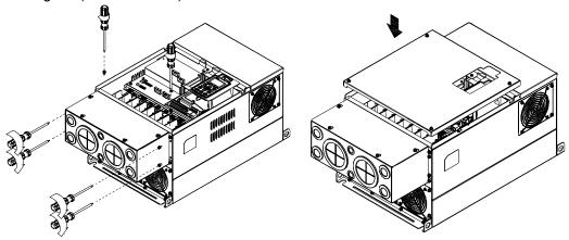
3. Fasten the 4 screws shown in the following figure. Screw torque:12~15kg-cm (10.4~13lb-in) \_ \_ \_ \_
