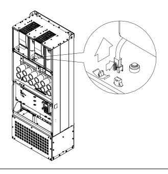
(4) Loosen the screw and remove the fan. Make sure fan power is properly disconnected before removal. Screw torque: 24~26kg-cm (20.8~22.6lb-in).
