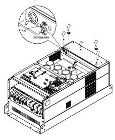
(4) Lift the fan by putting your fingure through the protective holes, as indicates in 1 and 2 on the figure.
