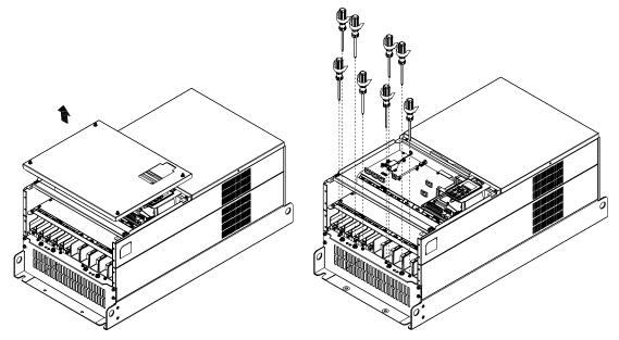
2. Install the conduit box by fastening all the screws shown in the following figure. Screw torque: 25~30kg-cm (20.8~30lb-in); Screw torque: 12~15kg-cm (10.4~13lb-in)
