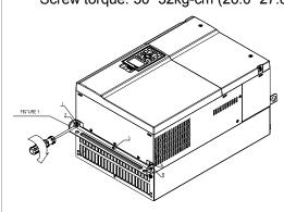
5. Fasten 4 screws (as shown in the following figure). Screw torque: 24~26kg-cm (20.8~22.6lb-in).
