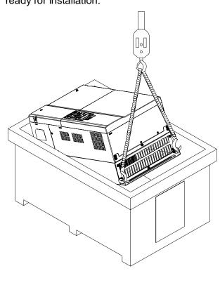
Loosen the 10 screws on the pallet, remove the wooden plate.
