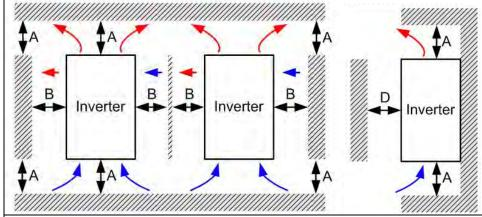
Multiple drives side-by-side installation and in rows (Frame A,B,C)
