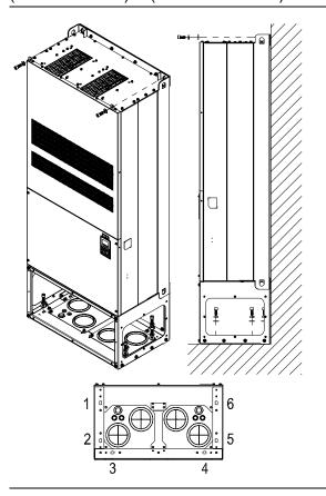
Secure the drive from the internal.
