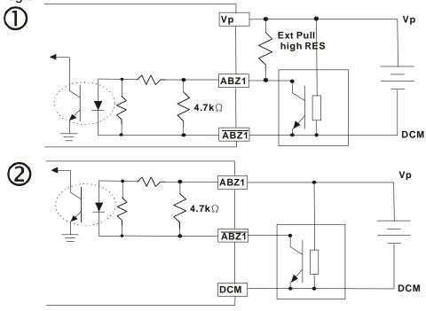
When wiring in this way, if there  $\,$  a signal on EMC-PG01's A1, B1 and Z1,LED lights is OFF.
