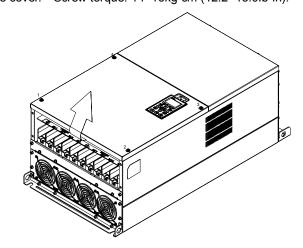
(1) Loosen the screw (as shown in figure below) and removes the cover. Screw torque: 14~16kg-cm (12.2~13.9lb-in).
