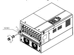
4. Fasten 5 screws (as shown in the following figure). Screw torque: 30~32kg-cm (26.0~27.8lb-in).
