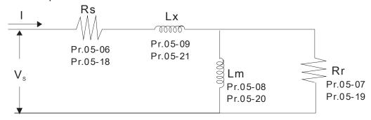
If Pr.05-00 is set to 2 (static test), user needs to input the no-load current value of motor into Pr.05-05 for motor 1/Pr.05-17 for motor 2.
