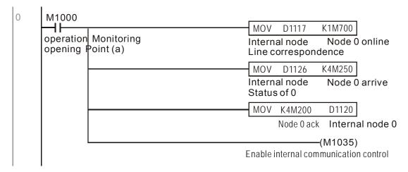
Diagram 2: When Slave 1 on-line status is detected, it will delay for 3 seconds before control command is enabled.
