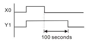
When input X0 is ON, output coil Y1 will be ON at the same time due to the corresponding normally close contact OFF makes timer T10 to be OFF. Output coil Y1 will be OFF after delaying 100 seconds (K1000\*0.1 seconds = 100 seconds) once input X0 is OFF and T10 is ON. Please refer to timing chart above.
