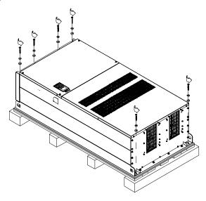
Lift the drive by hooking the lifting hole. It is now ready for installation.
