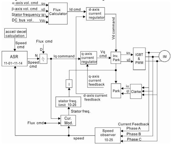
When setting Pr.00-11 to 6, PM FOC sensorless control diagram is shown as follows:
