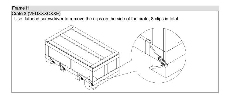
Remove the crate cover, EPEs, rubber and manual.
