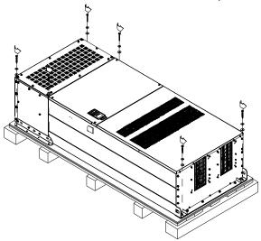
Loosen 6 of the M6 screws on the side and removes the 2 plates, as shown in following figure. The removed screws and plates can be used to secure AC motor drive from the external.
