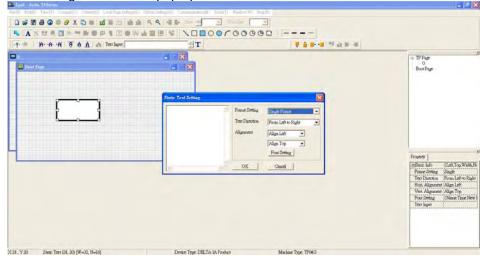
On the right hand side of the Static Text Setting, you can adjust the frame setting, the text direction, the alignment and the font setting. Once you finish all the adjustments that you need. You can continue to input your text in the blank space of Static Text Setting window. When you finish inputting your text, click on OK to continue your next step or click cancel to abort the current step.
