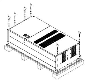
Loosen 6 of the M6 screws on the side and remove the 2 plates, as shown in below. The removed screws and plates can be used to secure the AC motor drive from the external.
