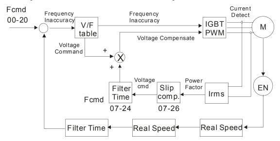
When setting Pr.00-11 to 2, the sensorless vector control diagram is shown as follows.
