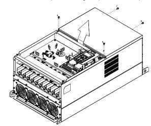
(3) Loosen the screws and remove the fan. (As shown in the figure below) Screw torque: 24~26kg-cm (20.8~22.6lb-in).
