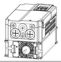
2. Disconnect the power terminal before removing the fan.
