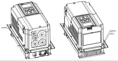
4. Plate installation, place 4 of the screw 2 (M6) through accessory 2&3 and the plate then fasten the screws. Screw torque: 25~30kg-cm (5.21~6.94lb-in).
