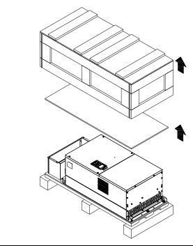
Loosen the 9 screws on the pallet and remove the wooden plate.
