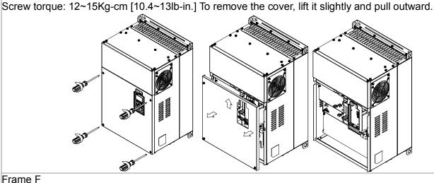
Screw torque: 12~15Kg-cm [10.4~13lb-in.] To remove the cover, lift it slightly and pull outward
