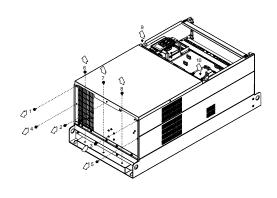
(3) Loosen screw 1,2,3 and remove the protective ring (as shown in figure below) Screw torque: 15~20kg-cm (12.2~13.9lb-in).
