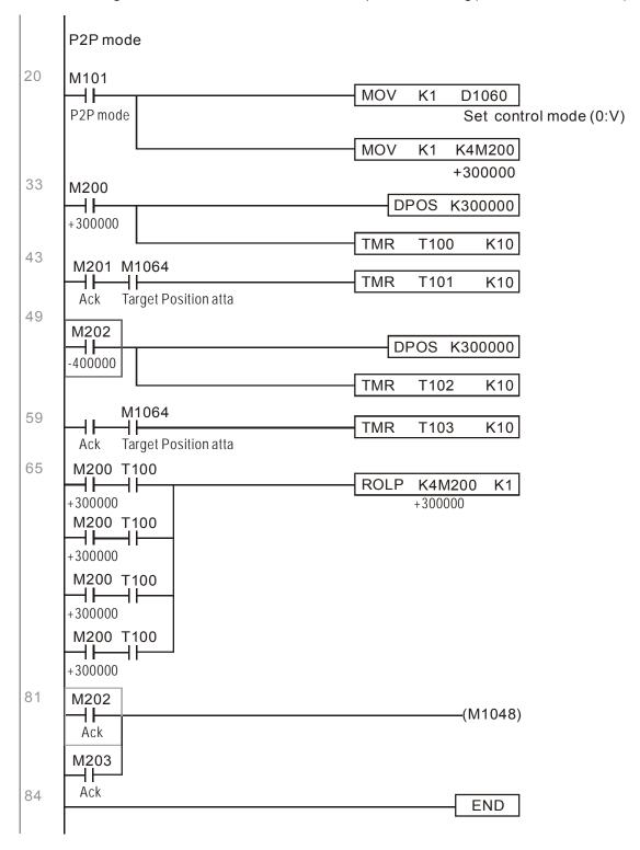
If user's application does not require homing action, you may skip Part I and Part II and go to the next step. In this example, turn AC motor drive power ON by trigger X2 and set M1002 to position mode, then the PLC program will be in position mode when drive power turns ON.
