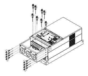
Fasten all the screws. Screw torque: 25~30kg-cm (20.8~30lb-in).
