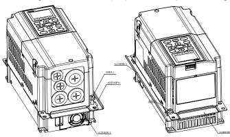
3. Install accessory 2&3 by fastening 2 of the screw 2(M6). Screw torque: 25~30kg-cm (5.21~6.94lb-in).
