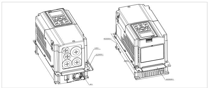
2. Install accessory 1& 2 by fastening 2 of the screw 1(M3). Screw torque: 25~30kg-cm (5.21~6.94lb-in). (As shown in following figure)
