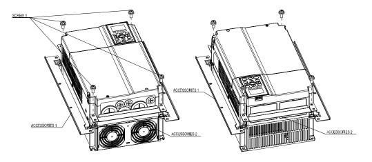
2. Plate installation, place 8 of the screw 2 (M6) through accessories 1&2 and the plate then fasten the screws. Screw torque: 25~30kg-cm (5.21~6.94lb-in). (As shown in the following figure)
