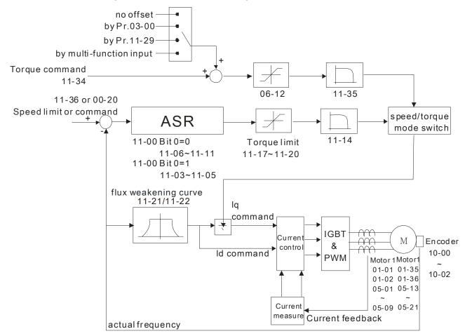
III TQC Sensorless control diagram is shown in the following:
