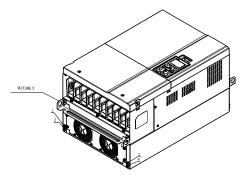
6. Fasten 5 screws (as shown in the following figure). Screw torque: 24~26kg-cm (20.8~22.6lb-in).
