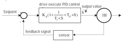
$K_p$ : Proportional gain(P)  $T_i$ : Integral time(I)  $T_{d}$ : Derivative control(D) S: Operator
