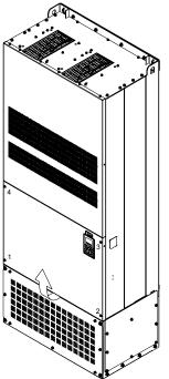
(2) Loosen the screw and remove the top cover. Screw torque: 24~26kg-cm (20.8~22.6lb-in).
