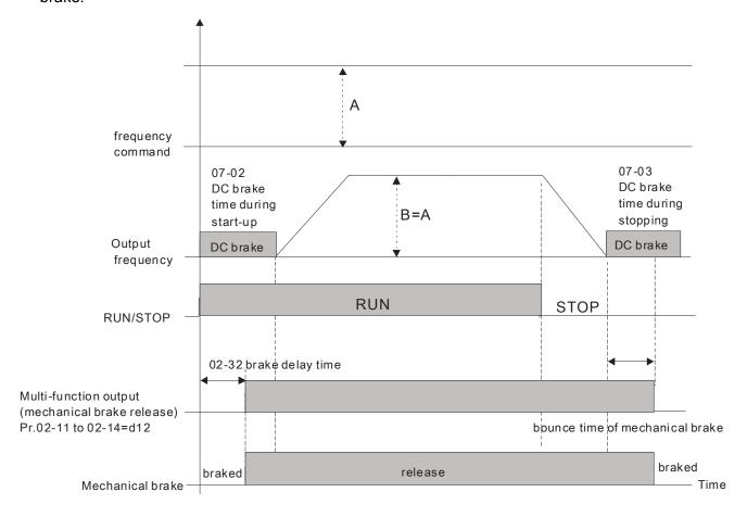
If this parameter is used without DC brake, it will be invalid. Refer to the following operation timing.
